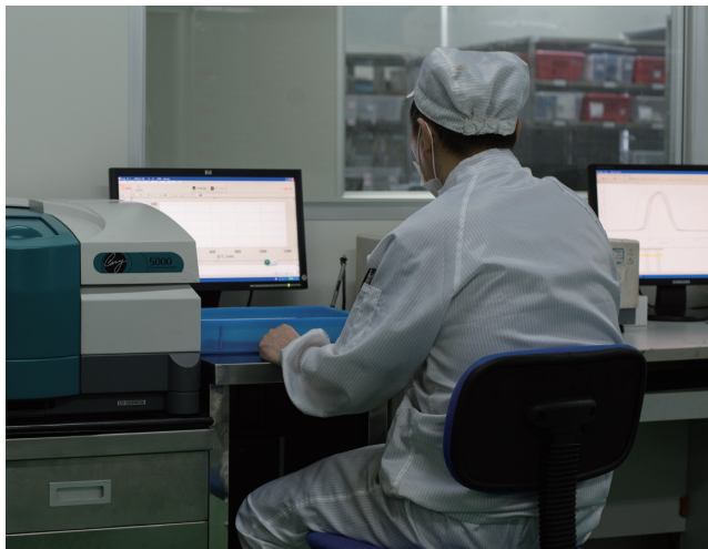
Cary 5000 Photospectrometer for measuring transmsion, OD6 of optical depth can be recognized
