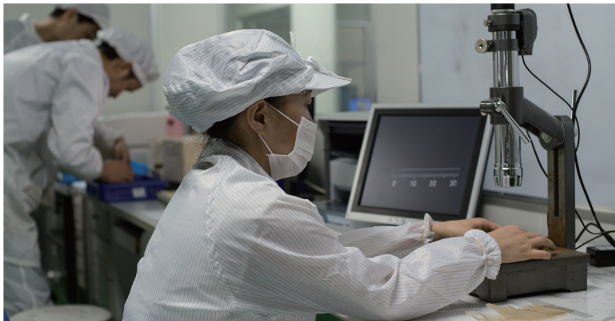
Collimator for testing cubes beam deviation
